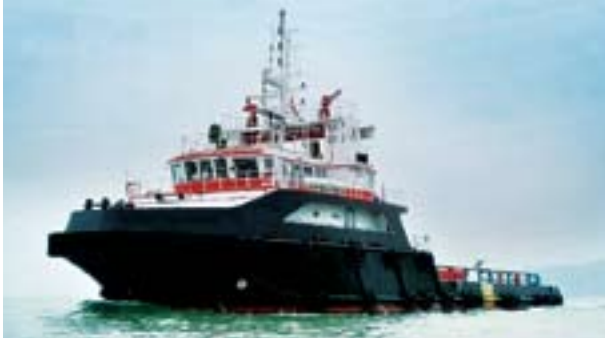
Anchor Handling Tug (AHT)
